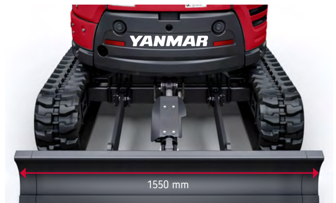
Extended: increased stability for improved digging and loading performances
