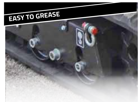
Greasing the undercarriage is easy and fast: nothing has to be taken apart.
