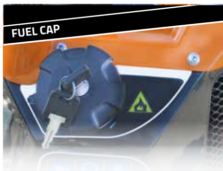
the diesel machine has a key protected fuel cap
