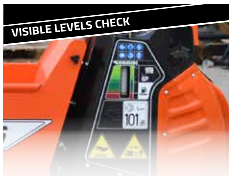
The window on the left side of the unit allow an immediate check of the fuel level
